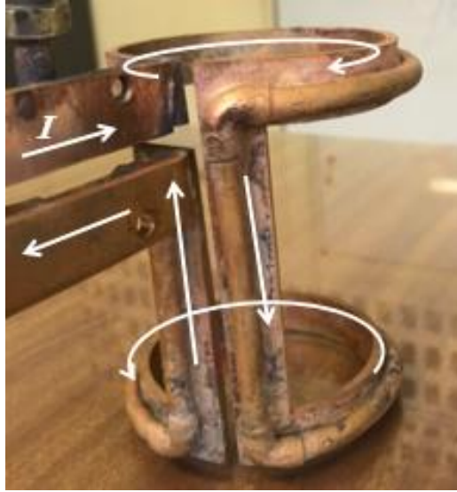
Figure 22: Anti-parallel double loop fabricated structure
