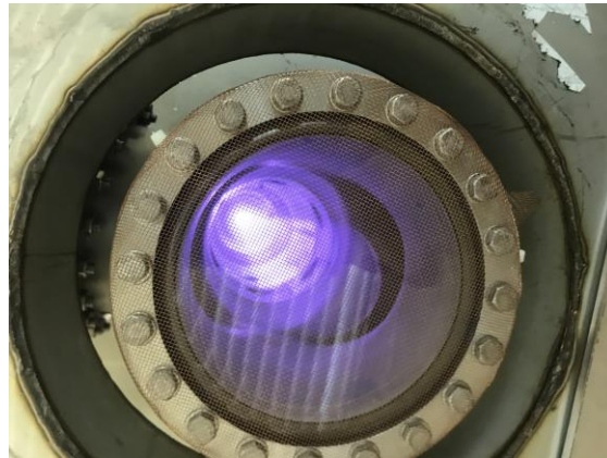
Figure 66: Blue mode plasma generation by the modified helix antenna installed on Polaris
