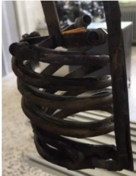
Figure 61: Modified helix fabricated antenna
