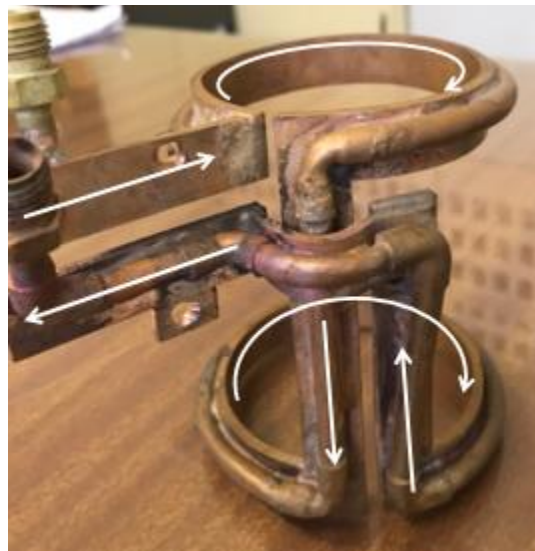
Figure 29: Parallel double loop fabricated antenna
