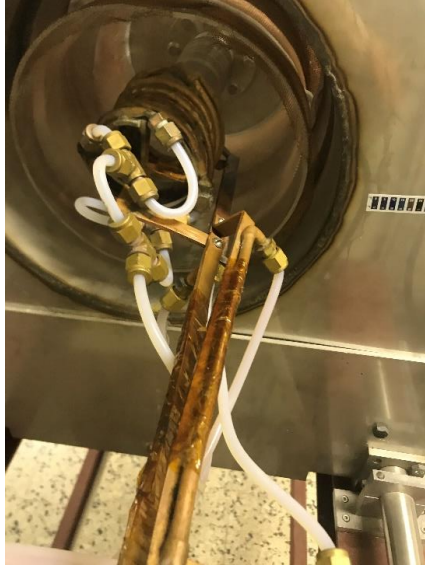
Figure 62: Modified helix antenna mounted on AUB's Lebanese Linear Plasma Device (Polaris)
