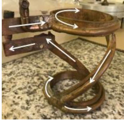
Figure 36: Fractional helix fabricated antenna
