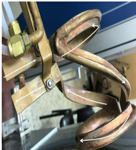
Figure 43: Parallel fractional helix fabricated antenna
