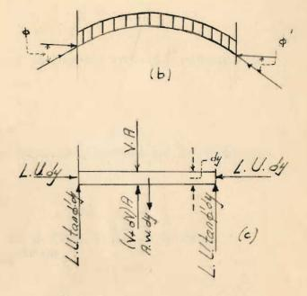
The weight of the granular material between the sections of y and y\*dy=A·w·dy; the total frictionam force acting upwards at the circumference will be L.U.tan ·dy; the total perpendicular pressure on the upper surface will be V.A: and the total pressure on the lower surface will be (V dV)A.
