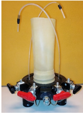
Figure 5.20 Latex membrane fitted over pedestal base
