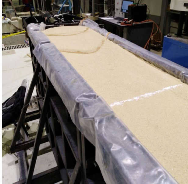
Figure 6.14 Formation of failure planes for the case of dense soil
