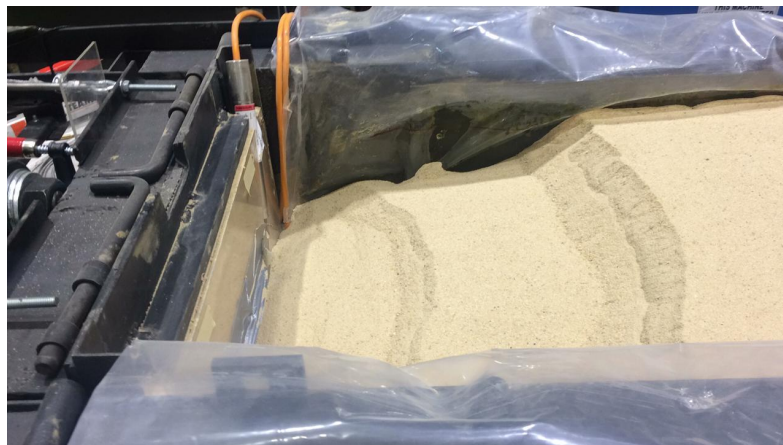
Figure 7.3 Soil cavity forming in front of the rigid wall during large active wall displacement
