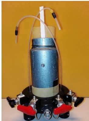
Figure 5.21 Split mold fitted around latex membrane
