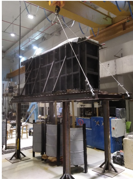
Figure 5.15 Emptying retaining system in storage barrels
