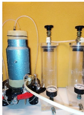
Figure 5.25 Vacuum drawn from within the sample
