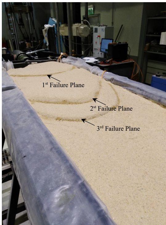
Figure 6.24 Failure planes formed in the experiment conducted on dense soil
