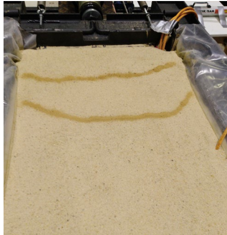
Figure 6.9 Surface traces of two failure planes forming in front of the wall in the medium-dense soil
