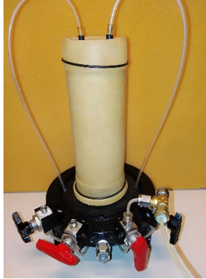
Figure 5.26 Soil sample with negative internal pressure
