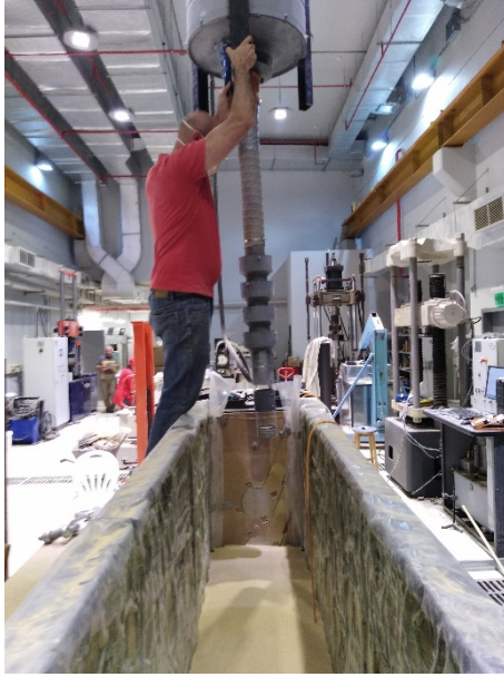
Figure 5.14 Filling the soil retaining system with sand using pluviation
