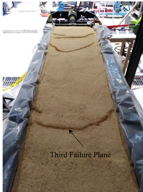
Figure 6.21 Formation of a 3 rd failure plane in response to three cyclic loading
