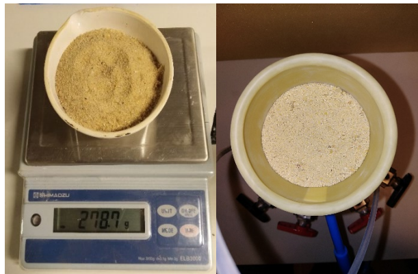
Figure 5.24 Dry sand weighed for the sampling of triaxial test
