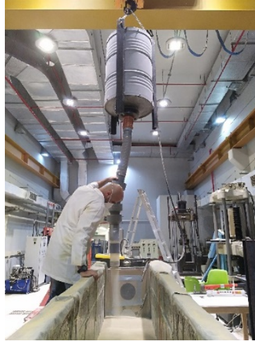
Figure 6.3 Filling the retaining system with granular soil using pluviation
