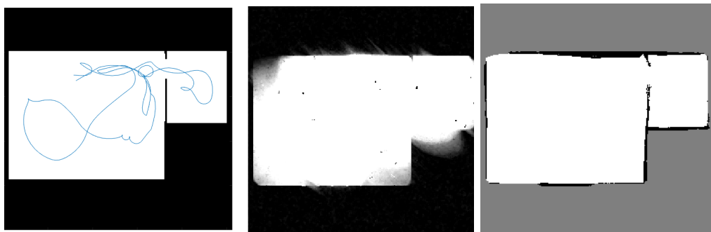
Figure 5.15: An example of an CAD map with a specific trajectory (left), the displacement field (middle), and its corresponding deformed image (right)
