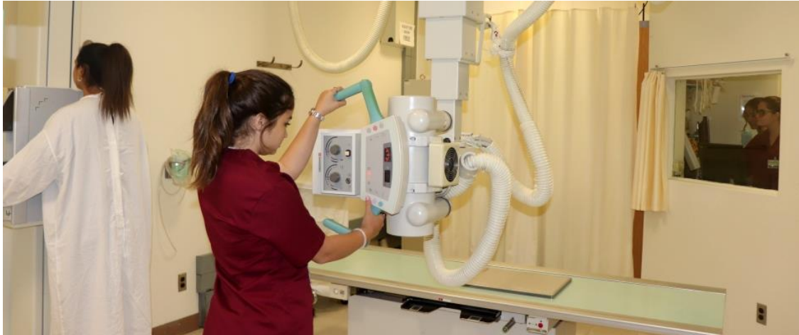
Figure 22 X-Ray medical machine employed for imaging of welded samples
