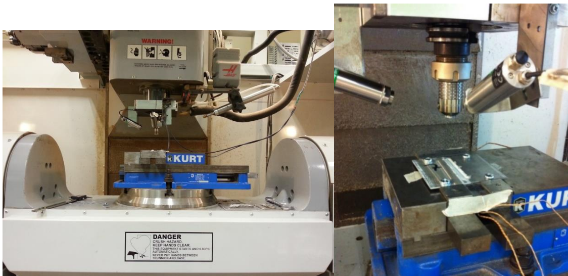
Figure 4 Experimental FSW setup
