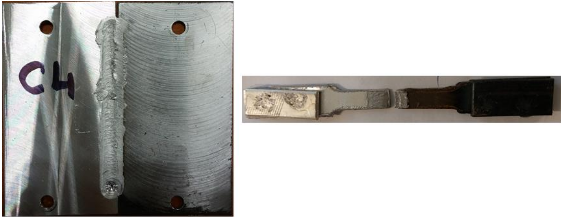
Figure 19 Sample C1 after welding and after tensile testing
