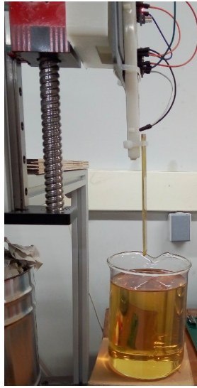
Figure 5.2: Experimental setup for viscosity measurement system
