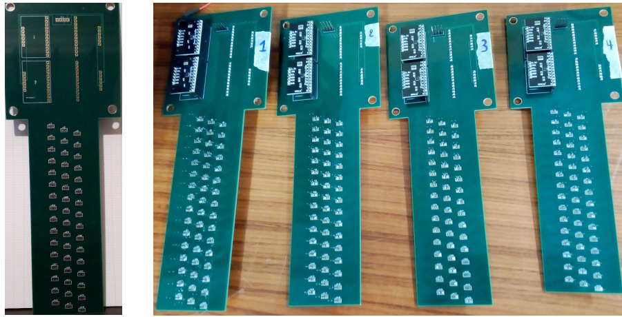
Figure 4.14: Implemented capacitive sensors - hand-held
