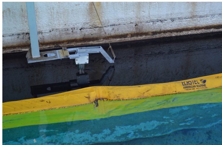
Figure 3.26: Capacitive sensing system mounted to the moving bridge
