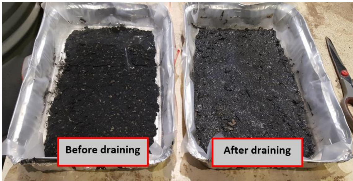
Figure 16 Loose cement mortars after 96 days of immersion in mQ (before and after draining the water)
