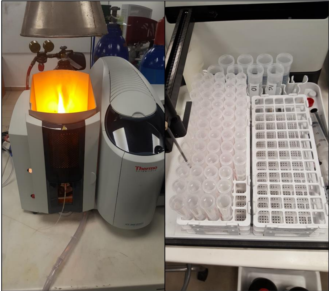
Figure 2 Analysis of samples using Atomic Absorption Spectroscopy
