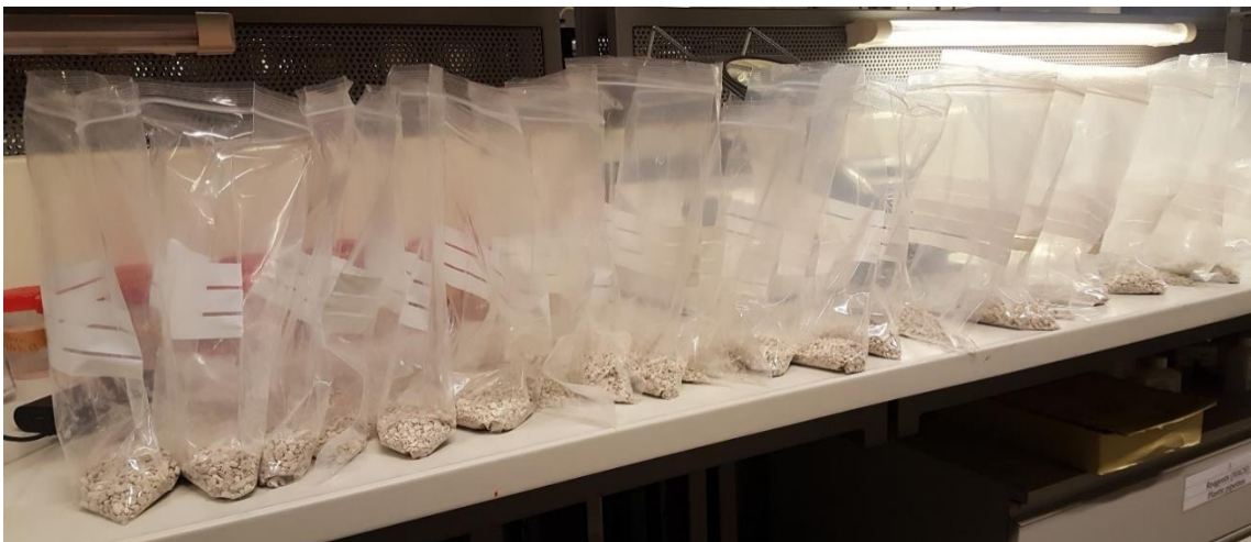
Figure 6 Mixing each mortar's components in a separate zip-lock bag in preparation of 50 x 50 x 50 mm cement cubes
