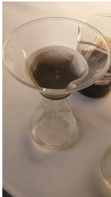
Figure 14 Filtering the solution after 24 hours to analyze the water sample
