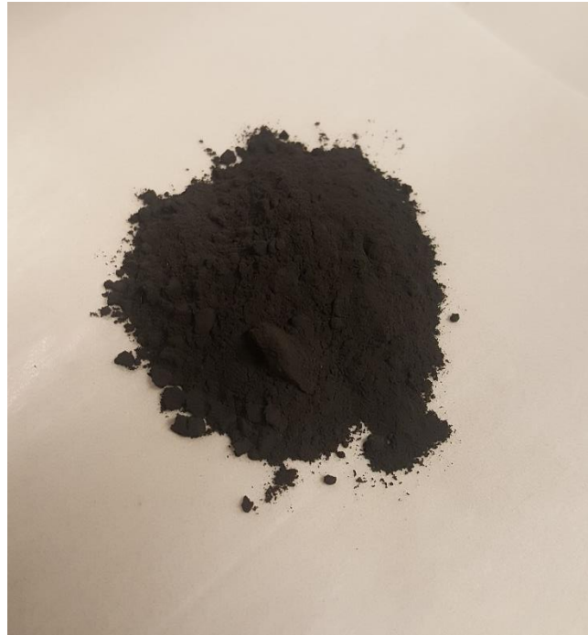
Figure 5 Fly ash used in the mixing of cement mortars
