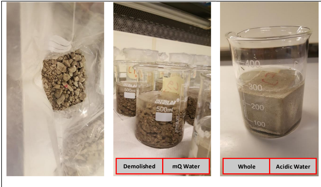
Figure 12 Immersion of demolished and whole control cement mortars for 24 hours in mQ and acidic water
