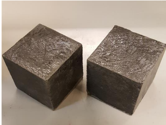
Figure 22 Cement mortars containing 10% replacement of fly ash from SICOMO
