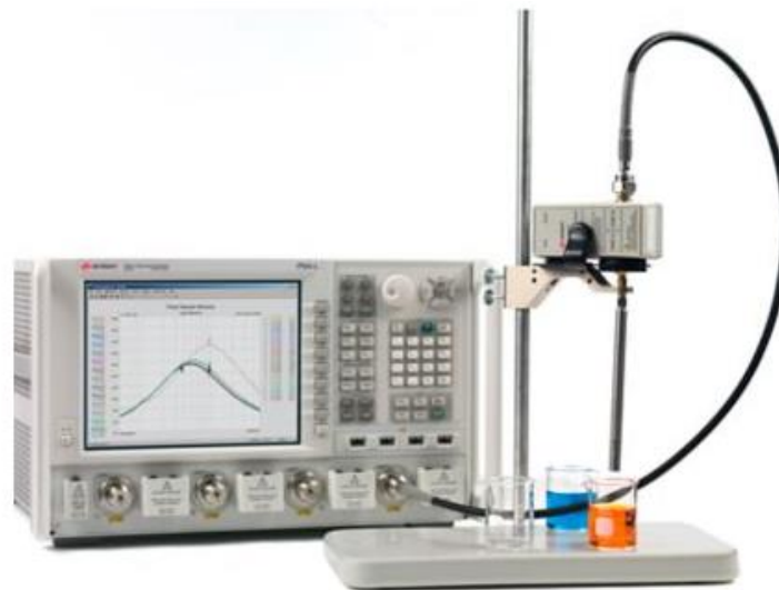
Figure. 27. A typical dielectric characterization kit with a VNA [38].
