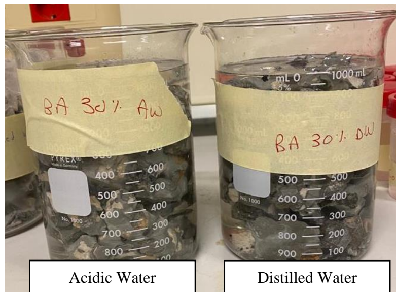
Figure 9: Rubble from pervious concrete containing 30% bottom ash immersed for 24 hours in 1000 ml acidic water and 1000 ml distilled water
