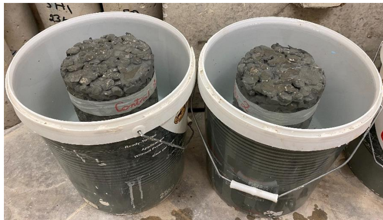
Figure 7: Pervious concrete cured in 11.85 liters of distilled water for 28 days
