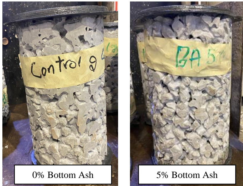
Figure 5: 150 mm x 300 mm capped pervious concretes containing 0% and 5% BA respectively
