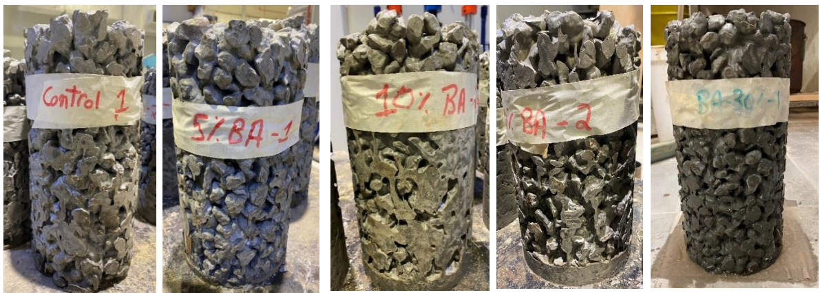
Figure 16: Pervious concrete cylinders with different BA percent replacement
