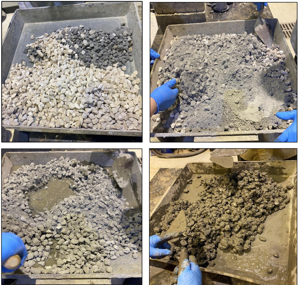
Figure 3: Hand mixing of 30% BA-based pervious concrete in a pan using limestone aggregates, bottom ash, cement and water
