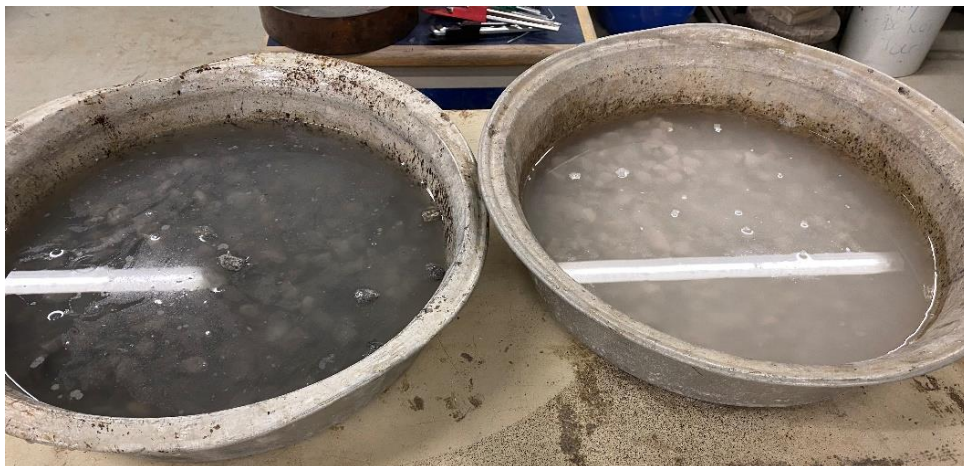
Figure 11: Specific gravity and water absorption for 12.5 mm control aggregates and 12.5 mm bottom ash
