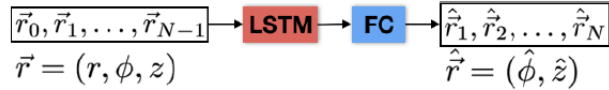
Figure 6.3: RNN hit predictor taking 3 hit coordinates as input and outputs a 2D next-hit prediction [57]
