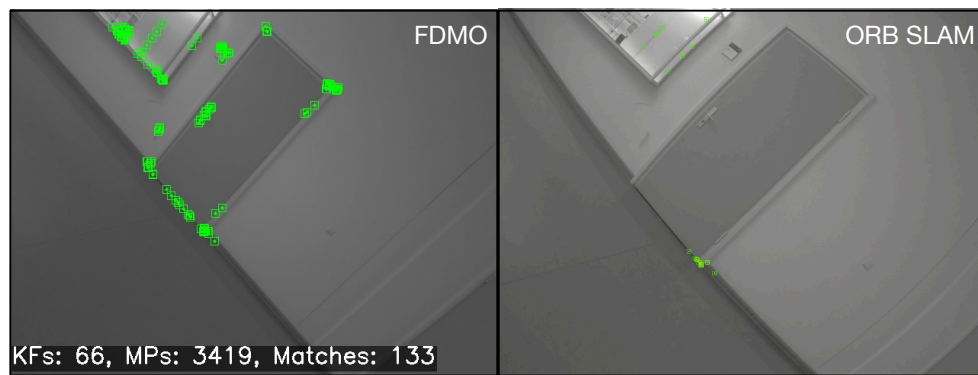
Figure 4.11: Features matched of FDMO (left) and ORB-SLAM2 (right) in a feature deprived environment (sequence 40 of the Tum_mono dataset).
