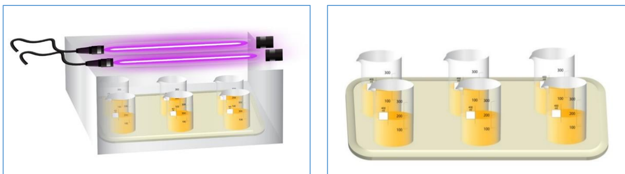
Fig. 4. Experimental Setup: six beakers are used as reactors for the performance of SMX removal in UVA/MIL-88-A/PS system where two UVA mosquito lamps are used for irradiating the solution from the top.
