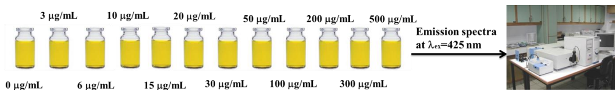
Figure 46 Schematic illustration of RNA sensing sample.
