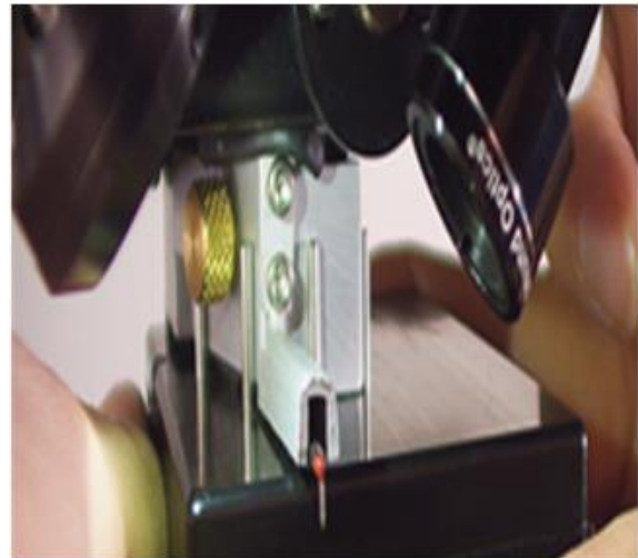
Figure 34: B- Type stylus of 2 \mu\text{m} size
