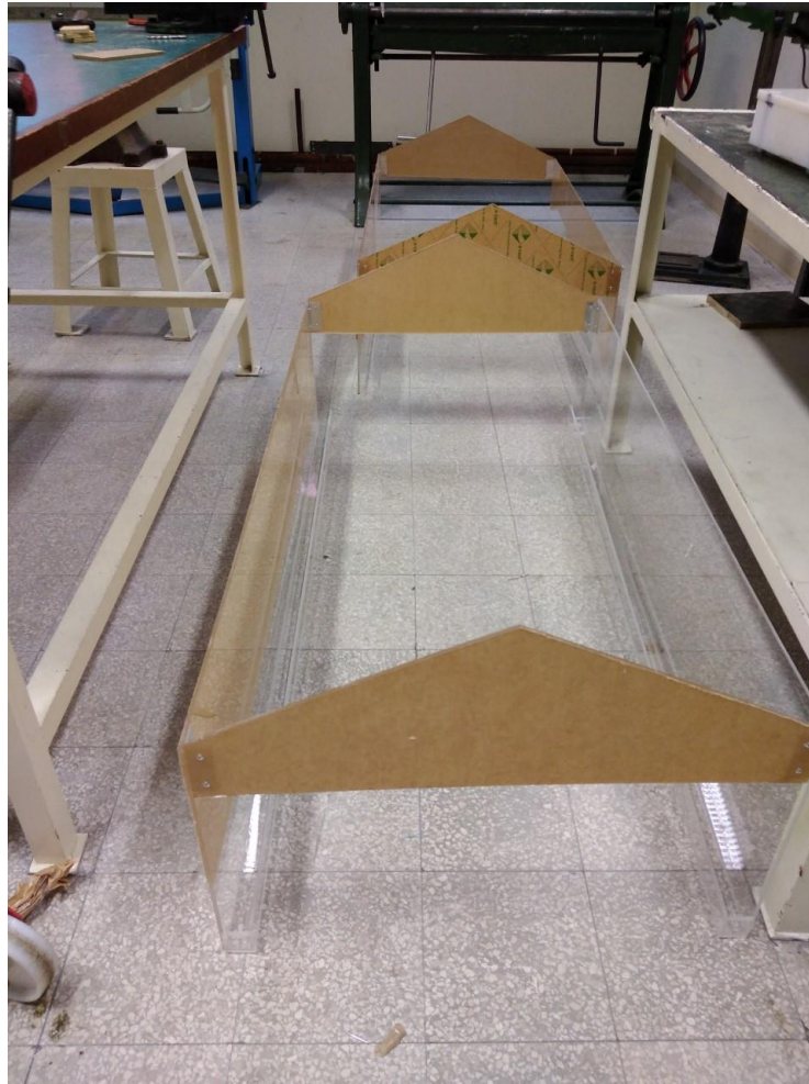
Figure 22: De- assembled parts of the set up (a): Smooth drum with basin, (b) Basin, (c) Rough drums, (d): Triangular glass cover
