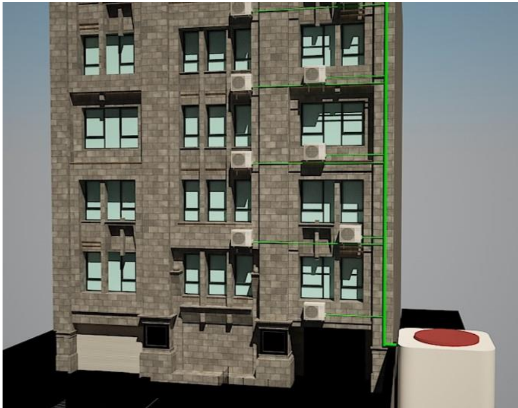
Figure 4. Proposed prototype of a retrofitted ACC water harvesting system on a residential building
