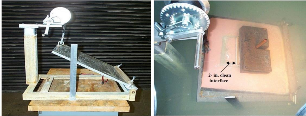
Figure 11. Tilt table frame and sliding of the plate at failure ( Najjar et al., 2007)
