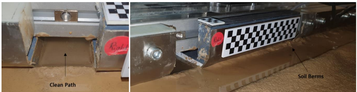
Figure 90. Soil berms around the setup and the created shearing path in Stage 3.
