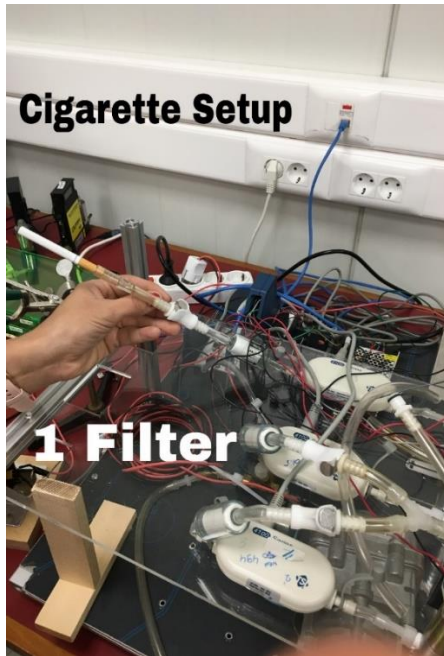
Figure 10: The setup of one single cigarette, designed in Dr. Alan Shihadeh Laboratory, connected to one filter attached to a programmed smoking machine linked to a software controlling the puffing parameters
