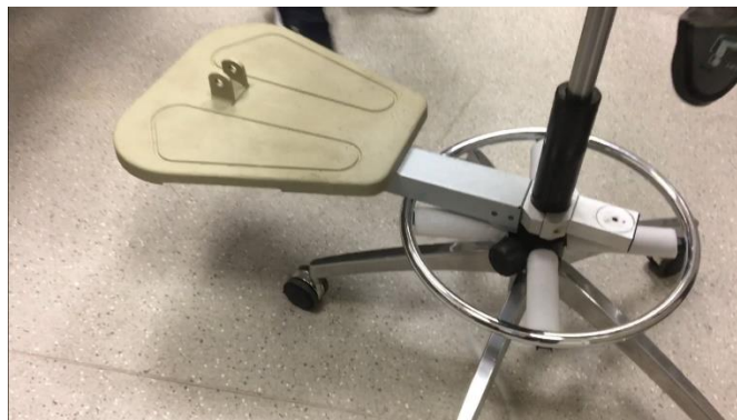
Figure 4 Modified chair with platform attached, serving as a footrest and providing space to place pedals.
