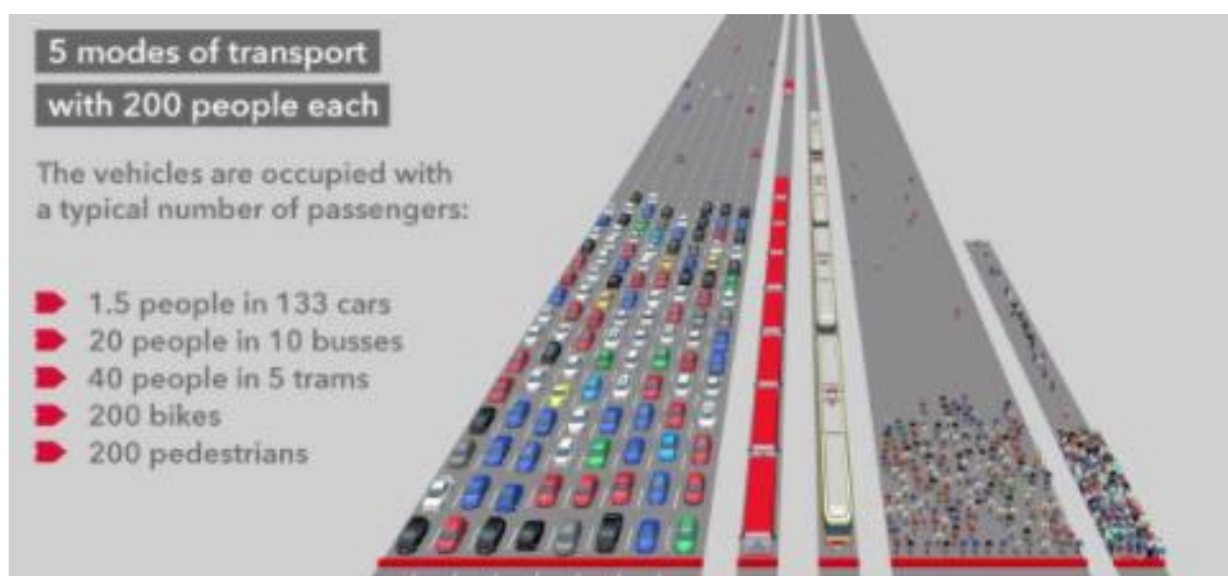
Figure 8-Space required by different transportation modes to carry 200 people Source: PTV Vision Traffic
