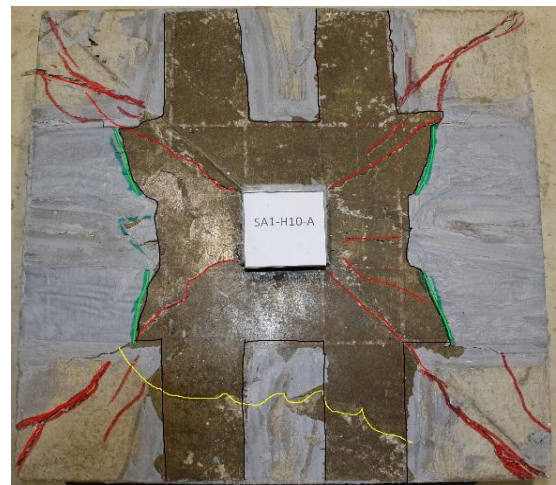
(c) Peeling off of the HFRP sheets in SA1-H10-A
