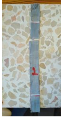
Figure 3.14 Mode of failure of the HFRP fabric strip
