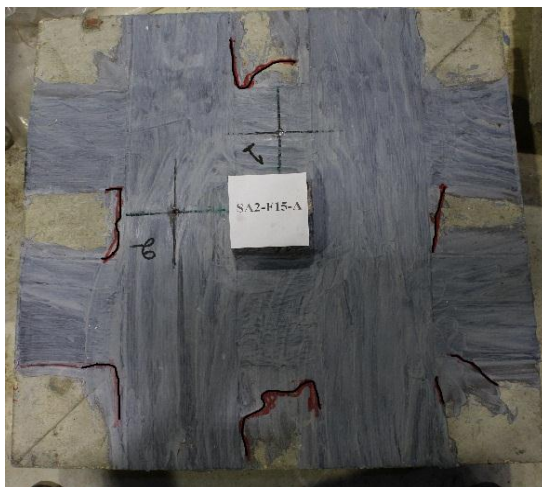
(a) Typical failure of specimens strengthened by CFRP
