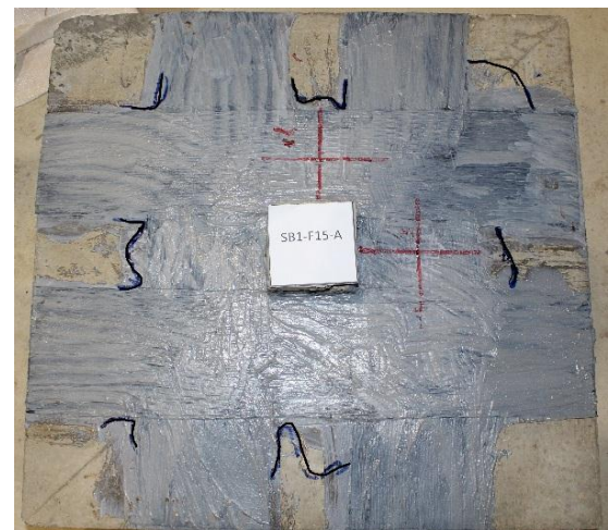
(a) Typical failure of specimens strengthened by CFRP
