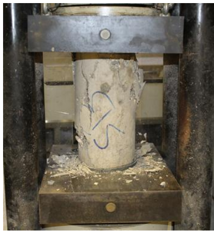
Figure 3.10 Test setup of the compression test of a concrete cylinder
