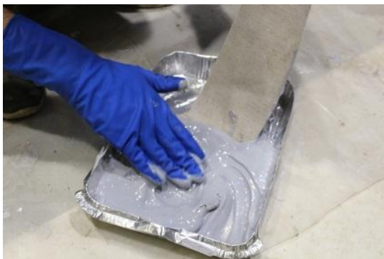
Figure 3.23 Saturation of the HFRP sheet with epoxy
