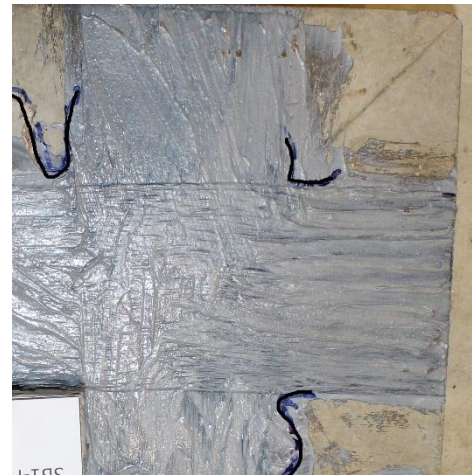
Figure 5.14 Comparison of crack patterns (a) SB1; (b) SB1-H15-A; and (c) SB1-F15-A
