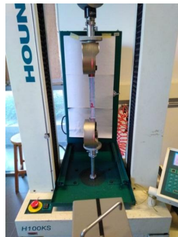
Figure 3.13 Tensile test setup of the HFRP fabric strips
