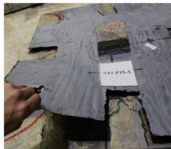
(c) Debonding of CFRP sheets in SA1-F15-A
