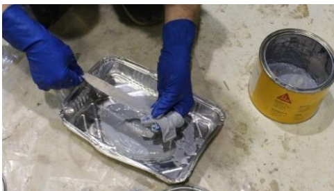
Figure 3.12 Preparation of the HFRP fabric strips for tensile testing
