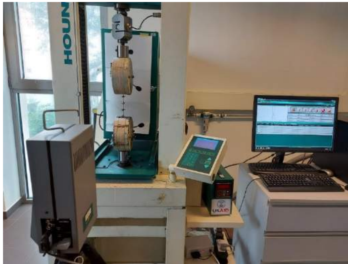
Figure 3.9: Tensile testing of the geogrid and bitumen textile sheets
