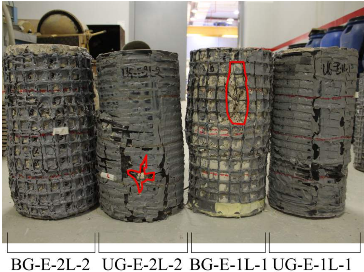
Figure 4.3: Failure modes of specimens externally confined using biaxial and uniaxial geogrid
