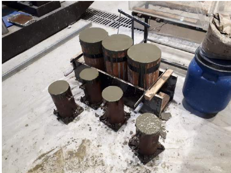
Figure 3.3: Pilot test cast specimens
