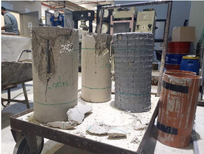
Figure 3.4: Pilot test specimens after testing
