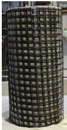
Figure 3.8: Bitumen coated E-glass textile
