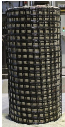
Figure 3.8: Bitumen coated E-glass textile
