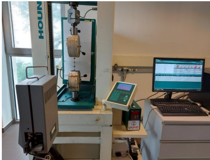
Figure 3.9: Tensile testing of the geogrid and bitumen textile sheets
