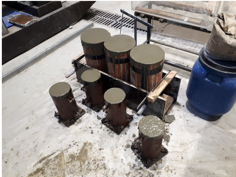
Figure 3.3: Pilot test cast specimens
