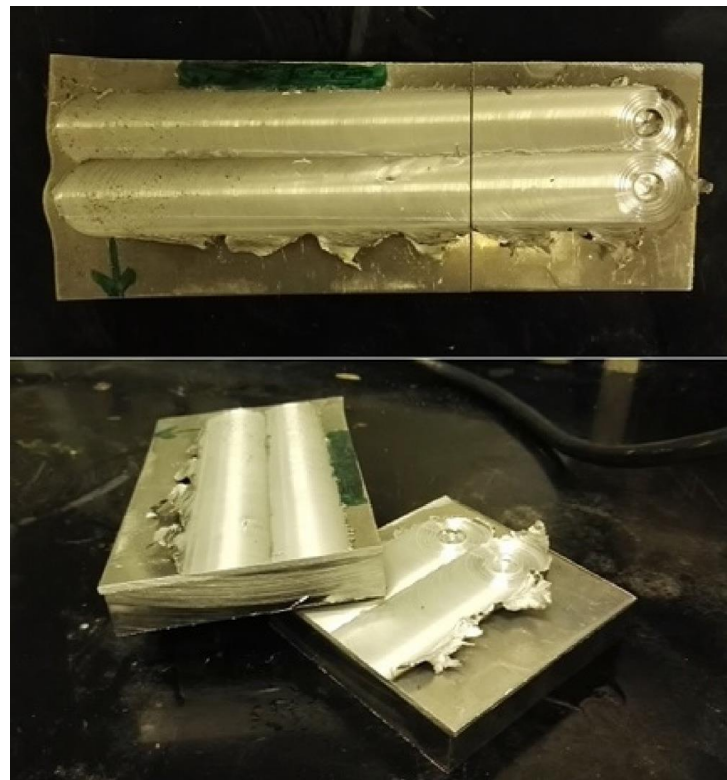
Figure 4.2. Two photographs of the top and cross-sectional views of a cut FSDC specimen with two cladding passes [159].
