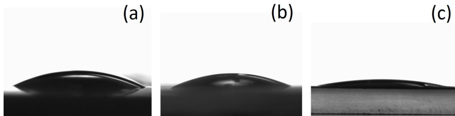
Figure 5.5: Contact Angle Drop Images of Polyimide Samples Treated with Ultraviolet-Ozone for (a) 15, (b) 30 and (c) 60 minutes.
