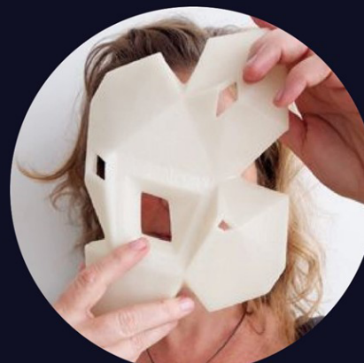
3D printed salt brick, Emerging Objects 8 parts salt : 1 part Maltodextrin
