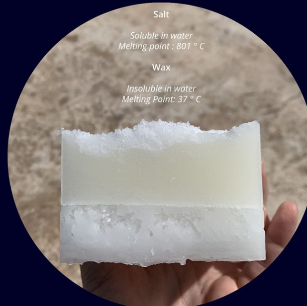
salt / wax brick layers of different compositions (top - fine grain salt, bottom - coarse grain salt)
