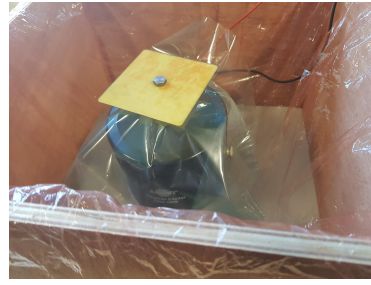
(b) Vibration Exciter with Protective Nylon Covers
