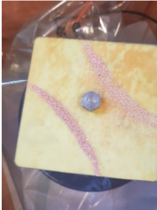
Figure 4.5: Copper powder shape benchmark.
