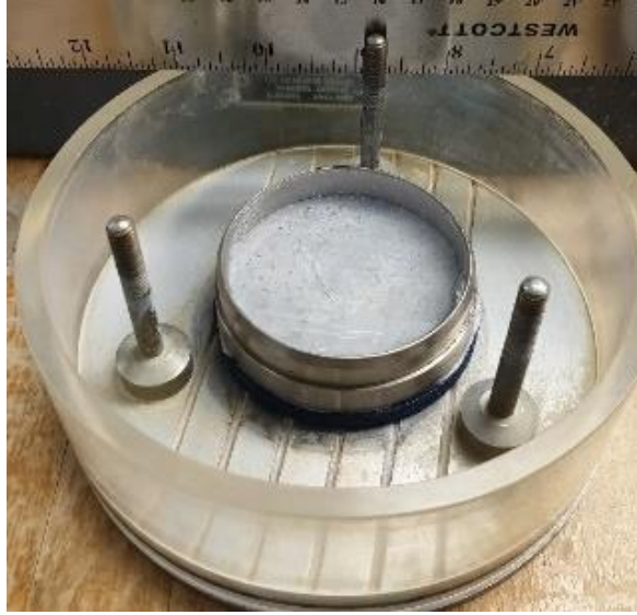
Figure 70: L4-S0.00 1-D consolidation sample in the odometer.
