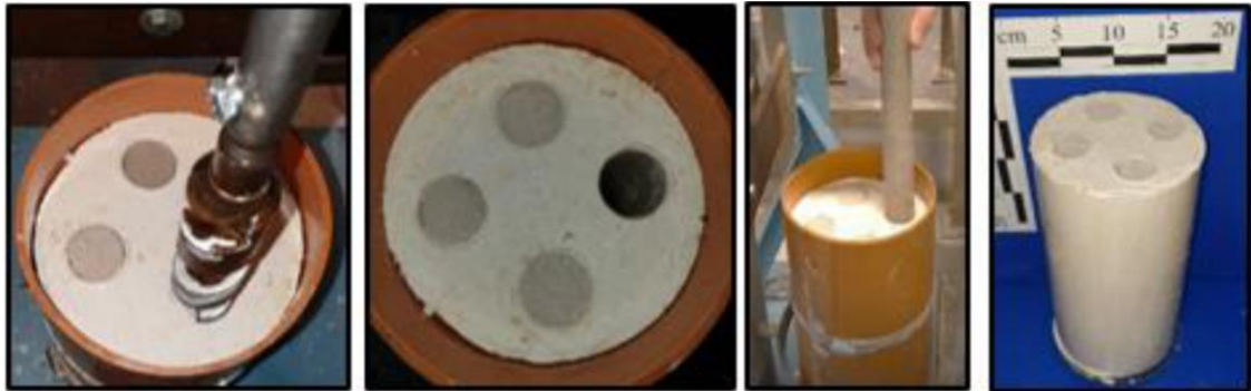
Figure 28: Drilling holes in kaolin specimen and sand column installation.
