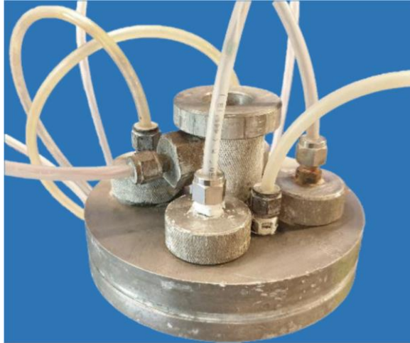
Figure 22: Side view of the upper cap showing the fittings and tubing to completely isolate the cell pressurized water from leaking towards the sensors and the specimens.
