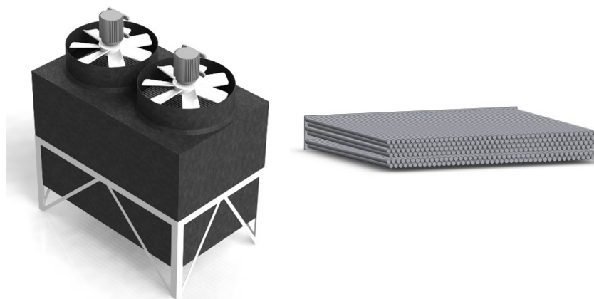
Figure 3 (a) SolidWorks Assembly File Containing all Individual Parts (b) Sample SolidWorks Part: Section of Tube Bundle
