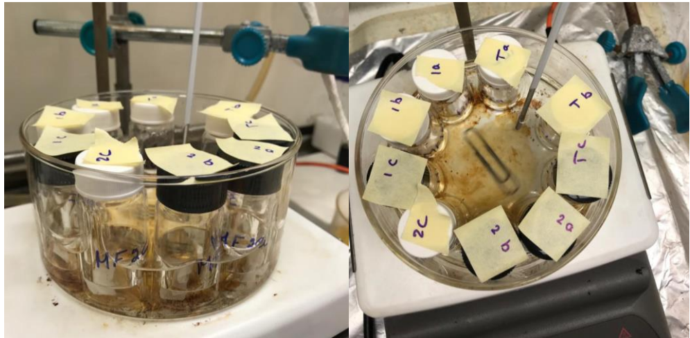
Figure 10: Modification setup of the PVC membrane in an oil bath
