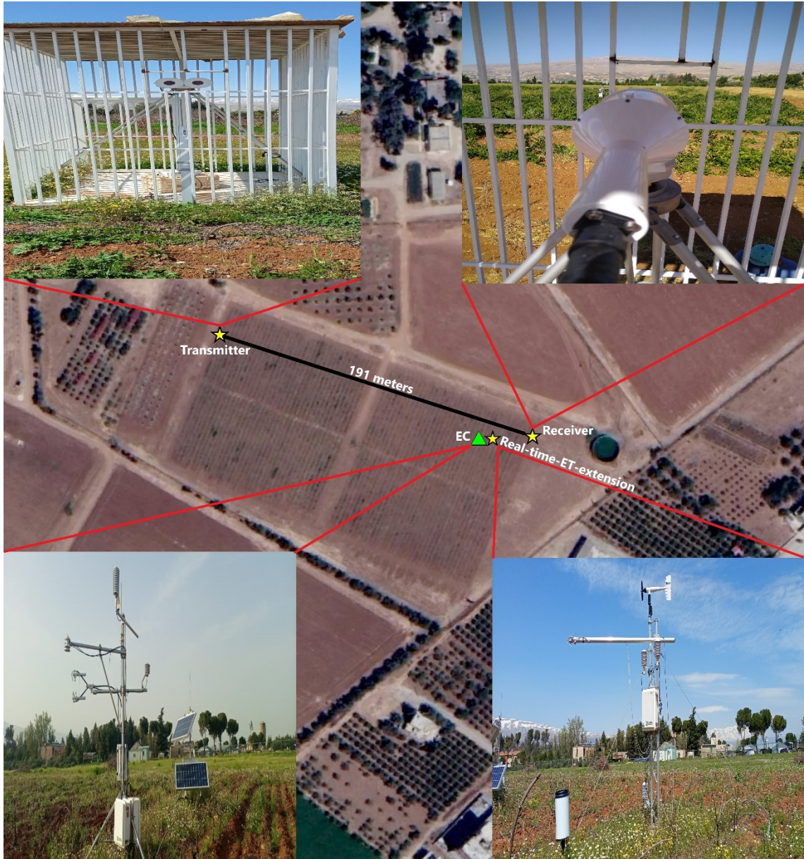
Figure 2: Layout of the deployed Boundary layer Scintillometer and Eddy Covariance system in the experimental site.
