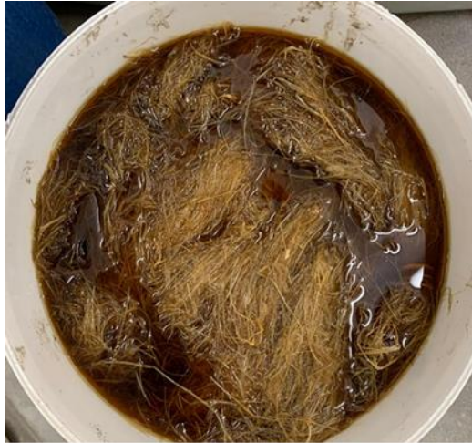
Figure 3.2 Hemp fibers in the sodium hydroxide solution
