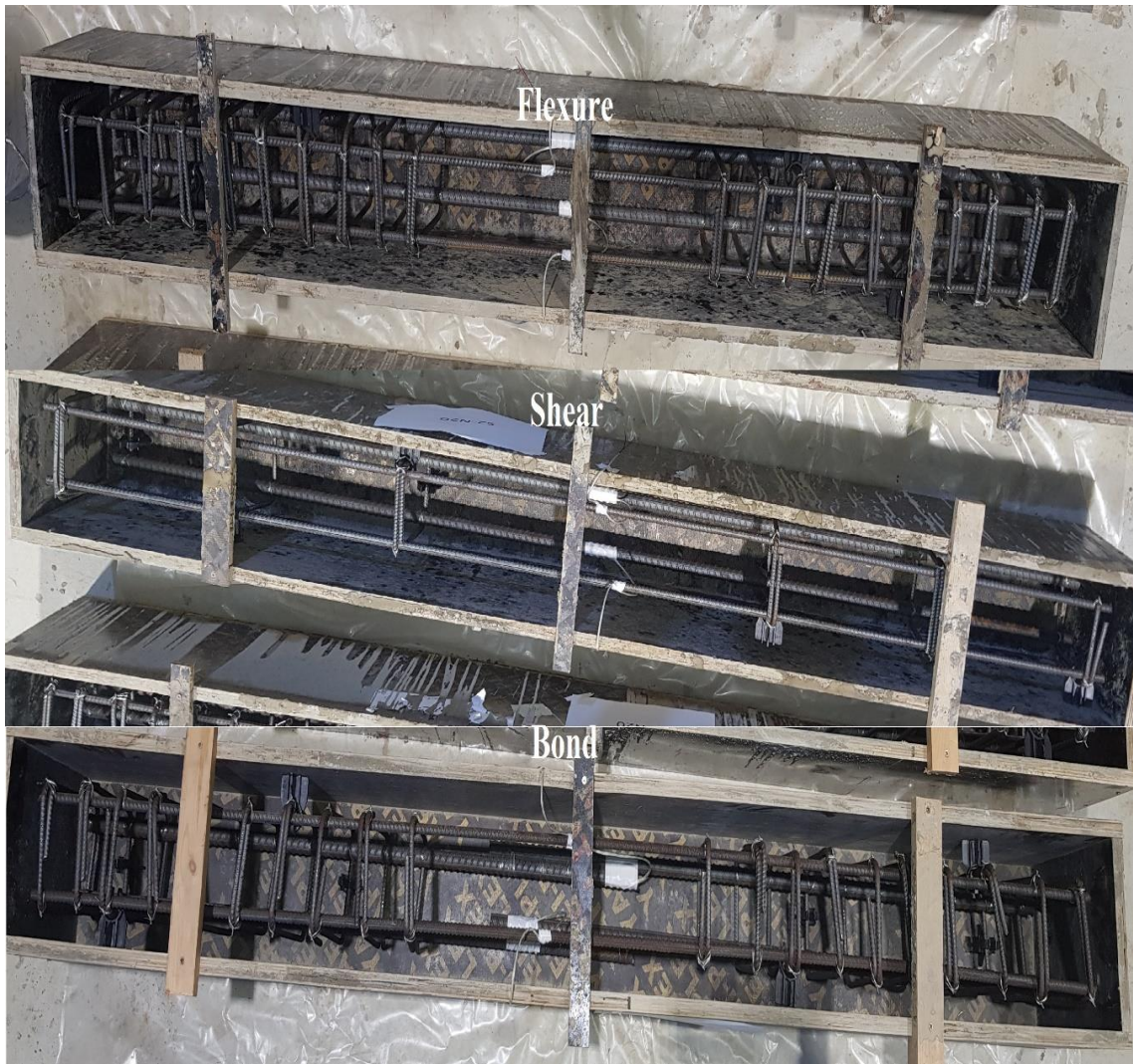
Figure 6.1 Typical reinforcement for each set of beams
