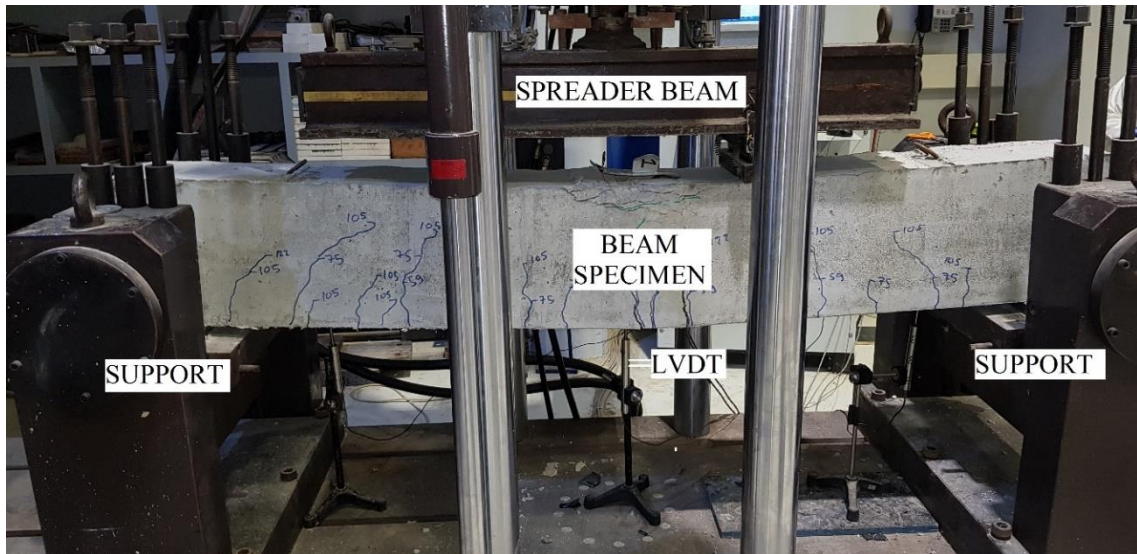
Figure 6.4 Actual view of the test setup for the beam specimens
