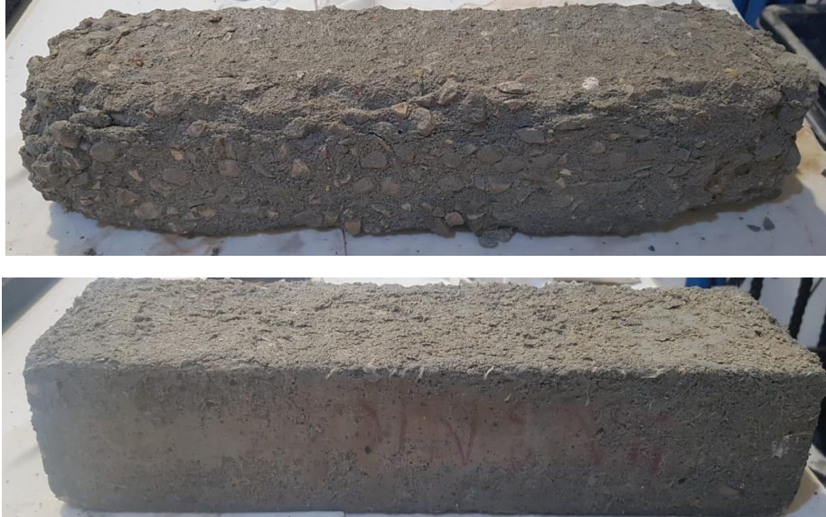
Figure 5.2 View of specimens R20 (top) and R10-H20-T1 (bottom) after 108 cycles.
