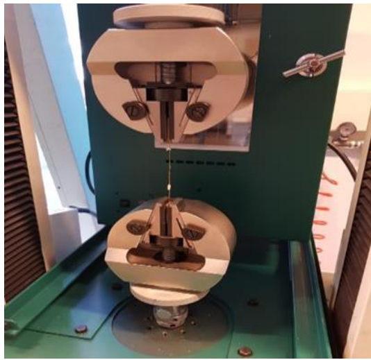
Figure 3.4 Hemp fiber mounted in UTM machine
