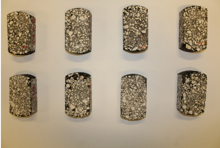
Figure 28 Briquette samples after sawing
