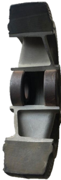
Figure 14: Depressurized tire: cross section view
