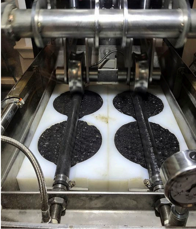
Figure 2: Asphalt Pavement Analyzer (AsphaltTesting, 2018)
