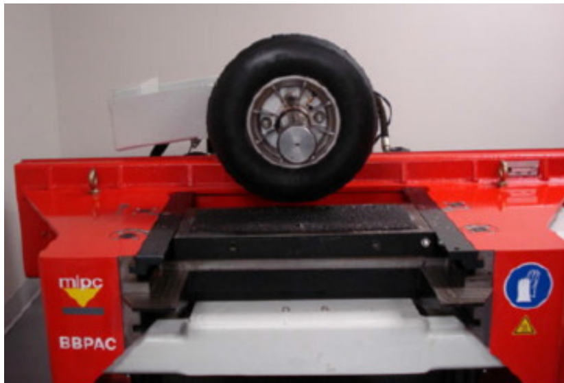
Figure 3: French rut tester (Saliani et al., 2021)
