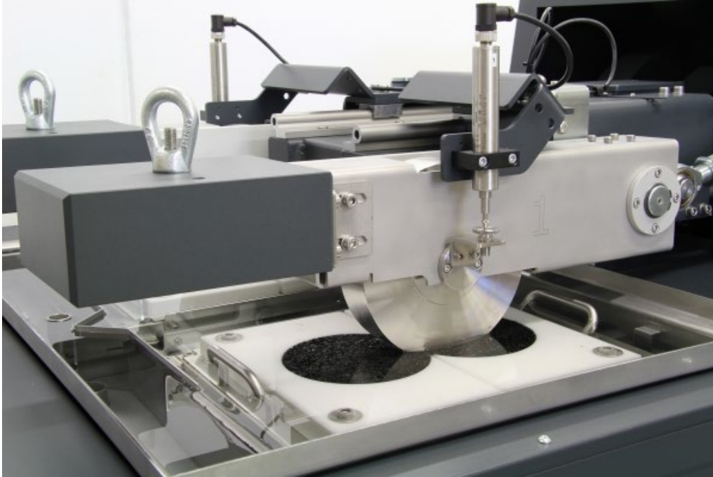
Figure 1: Hamburg wheel tracking tester (Geo Lab Nemo, 2017)
