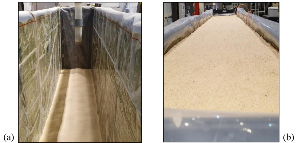
Figure 31. Horizontal sand bed during filling (a), Horizontal sand bed at the red mark at the end of filling (b)
