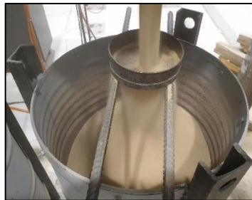
Figure 32. System placed on four jacks and ready for the emptying process (a), container under each valve (b), #4 sieves (c)
