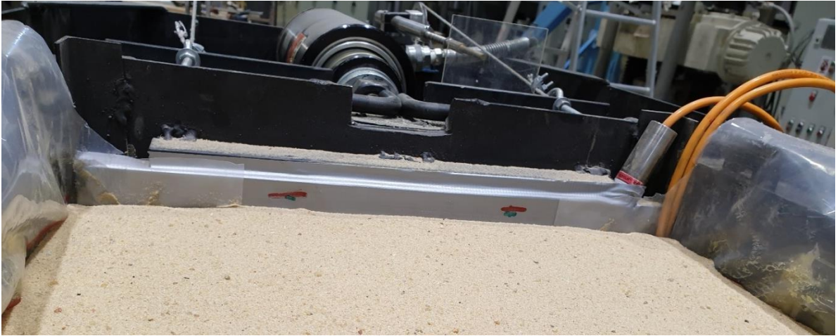
Surface level at the end of \pm 2 mm cycles, red marks the initial bed after filling tank at 1.2 m, and green marks the new level after the 1 st cycle \pm 2 mm cycle – test #1
