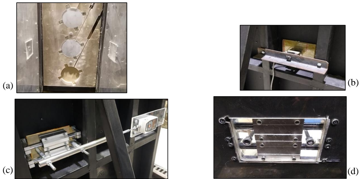
Figure 25. Low range force gauge and load cell mounted on opposite sides facing each other (a), load cell installed perpendicular to a block and flush with the inner face of the sidewall (b), force gauge parallel to a sliding block (c), sliding block flush with the inner face of the sidewall (d),
