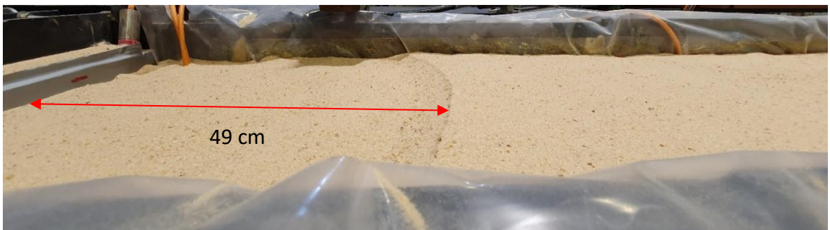
Bump at 49 cm away from the face of wall after 10 \pm 20 mm cycles – test #3
