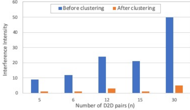
Figure 5.5: The effect of the number of D2D pairs on the interference intensity
