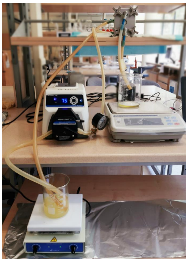
Figure 6 Pressure-Driven Oil-Water Separation (a) Schematic Setup and (b) actual lab setup
