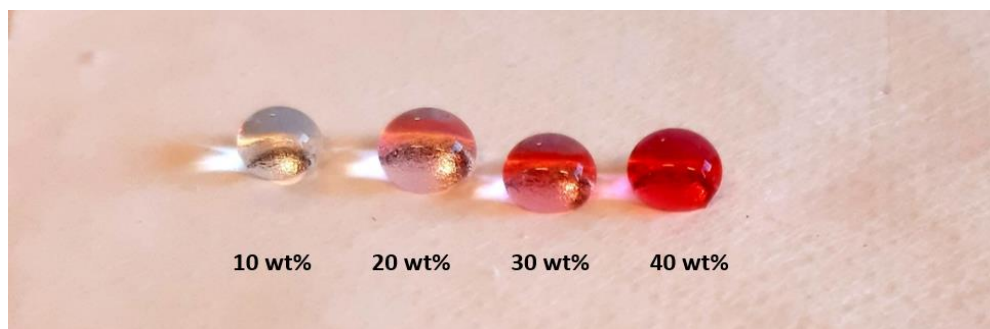
Figure 16. WCA on the electrospun membrane at various NaCL Concentrations
