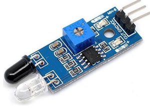
Figure 5.3: Infrared obstacle sensor module (RKI-3141)
