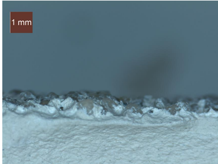
Figure 11. Microscopic view of a section across the oedometer sample showing the clay ( \sigma'_p=30\text{kPa} ) invasion into KAUST 20/30. Notice that invasion only reached one monolayer.
