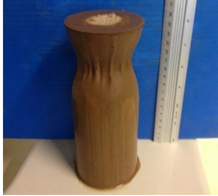
Figure 54. Necking failure for a clay sample reinforced with sand column
