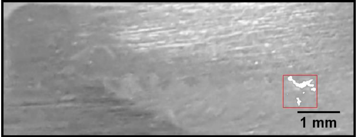
Figure 6 Photograph of the cross-section of weld sample 13 with the pin-hole defect highlighted in white with a red square marker; taken from Hamade and Baydoun [49].
