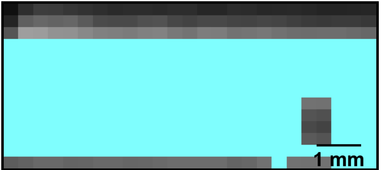
Figure 5 Segmented cross-section of weld case 13, showing the detected defect to the right; taken from Hamade and Baydoun [49].
