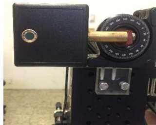
Fig.10: Four-quadrant photodiode detector used to measure both the transverse and longitudinal components of the vector angular deflection of the probe beam
