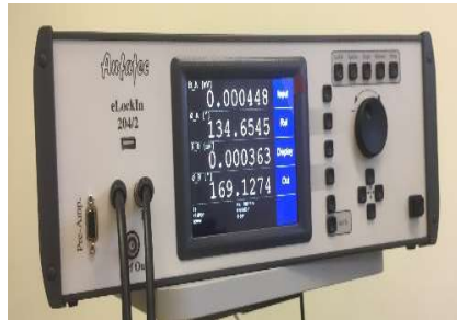
Fig. 11: Two-channel lock-in amplifier used in the developed setup.
