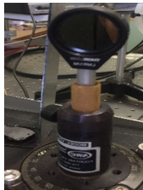
Fig.8: Biconvex ZnSe lens of 3 cm focal length used to focus the heating beam of the sample surface
