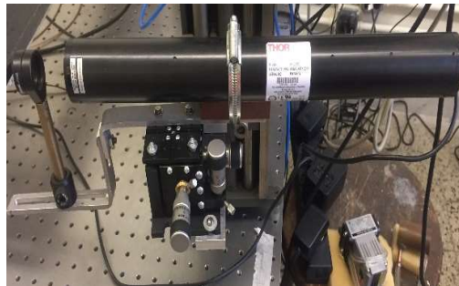
Fig.7: HeNe laser used in the experiment to generate the probe beam.
