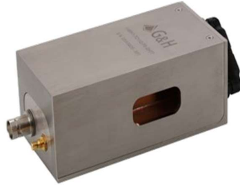
Fig.9: Acousto-optic modulator on the infrared heating beam
