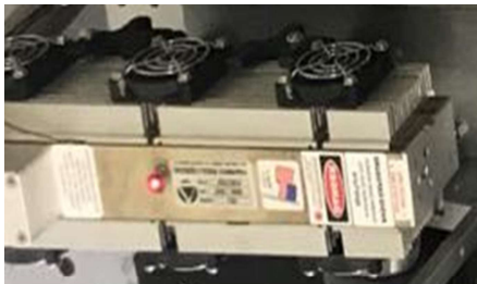
Fig.5: Picture of the pumping CO 2 infrared laser in the developed setup.
