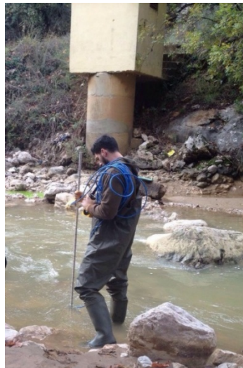
Figure 4-5. Discharge measurement using EM Flowmeter
