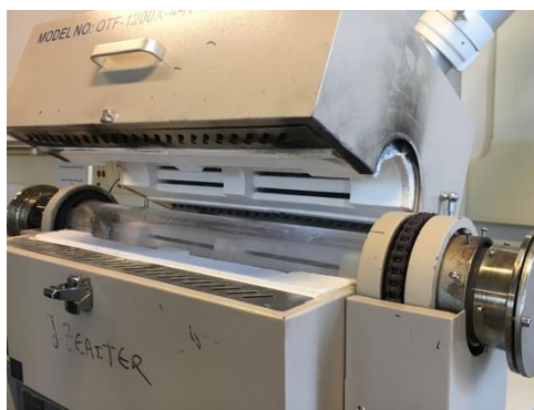
Figure 12 Large quartz cylinder placed inside circular heating sections
