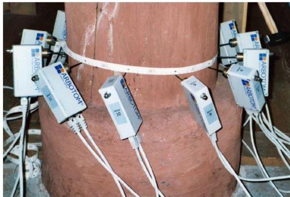
Figure 2.1 Sensor placement around the cross section of a specimen [5].
