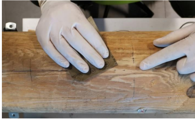
Figure 3.29 Smoothing the pole's surface with sandpaper before MFC coupling.
