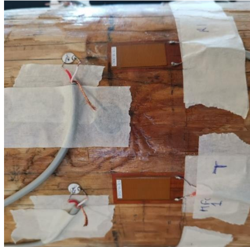
Figure 3.37 MFC – Timber impedance matching experiment.
