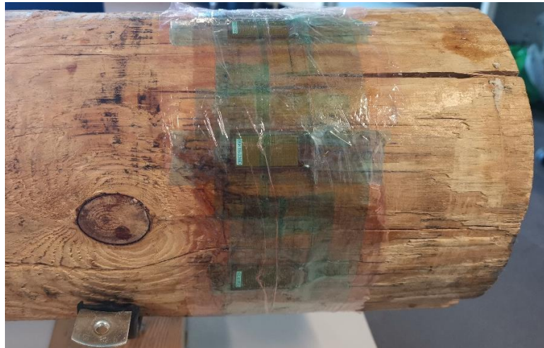
Figure 3.32 8-MFC Ring coupled around the circumference used for actuation.
