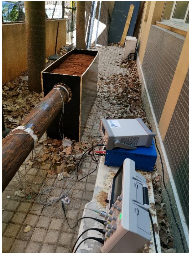
Figure 4.6 Experimental setup used on the 8-meter length timber utility pole.
