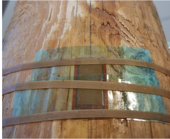
Figure 3.31 MFC coupled and pressed on one position of the pole's surface.
