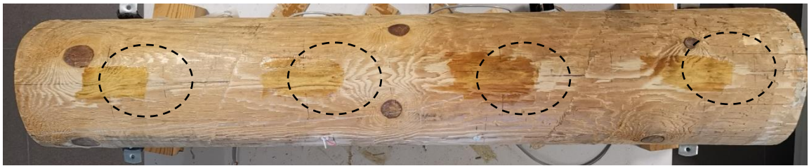
Figure 3.30 Dry thin layer of epoxy adhesive applied for additional smoothing.
