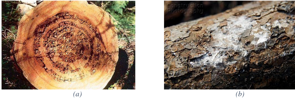
Figure 1.2 (a) Brown and (b) white rots in wooden poles.
