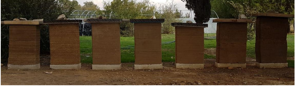
Figure 15 - Seven Rammed Earth Walls Constructed at AREC
