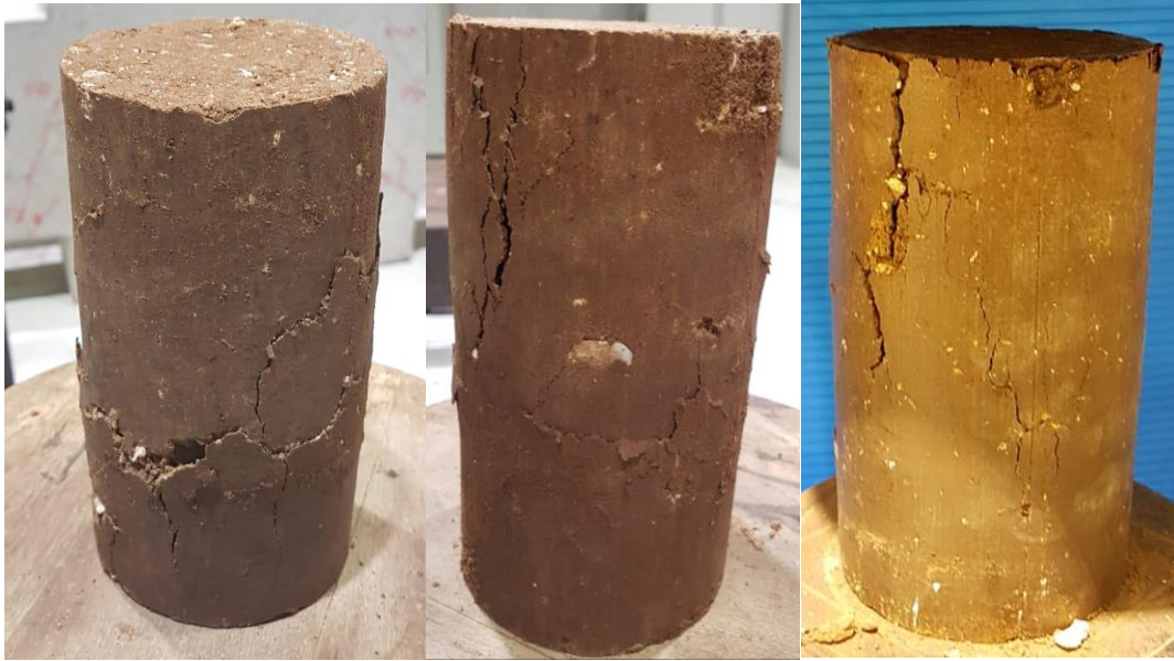
Figure 24 - Brittle Failure Cracking Pattern on Rammed Earth Compressive Strength Test Cylinders
