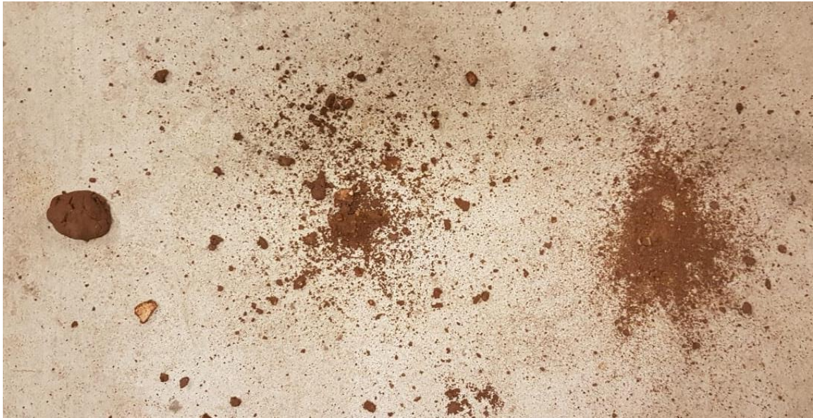
Figure 30 - Ball Drop Test Results with Decreasing Water Content from Left to Right
