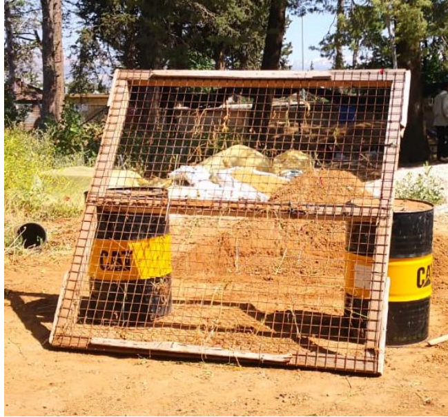
Figure 4 - Five-centimeter Sieve, On-site at AREC
