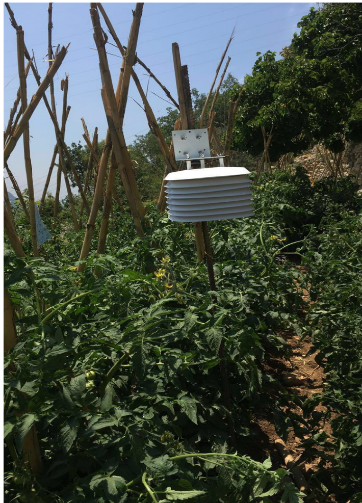
Figure 5. Data logger protected by a radiation shield
