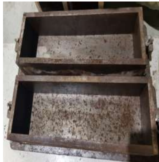
Figure 33. freeze and thaw mold (7.5x10x40.5 cm)
