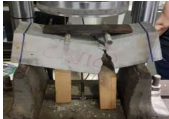
Figure 59. Flexural failure of mix without hemp
