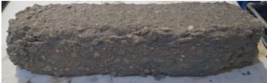
Figure 68. R20 and R10-H20-T1 specimens after 108 cycles
