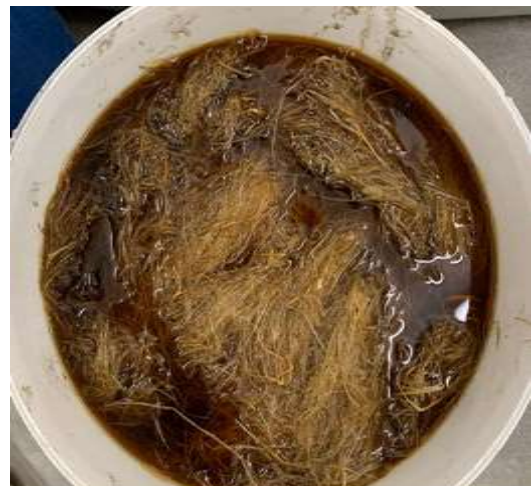
Figure 8. Hemp soaked in alkaline solution
