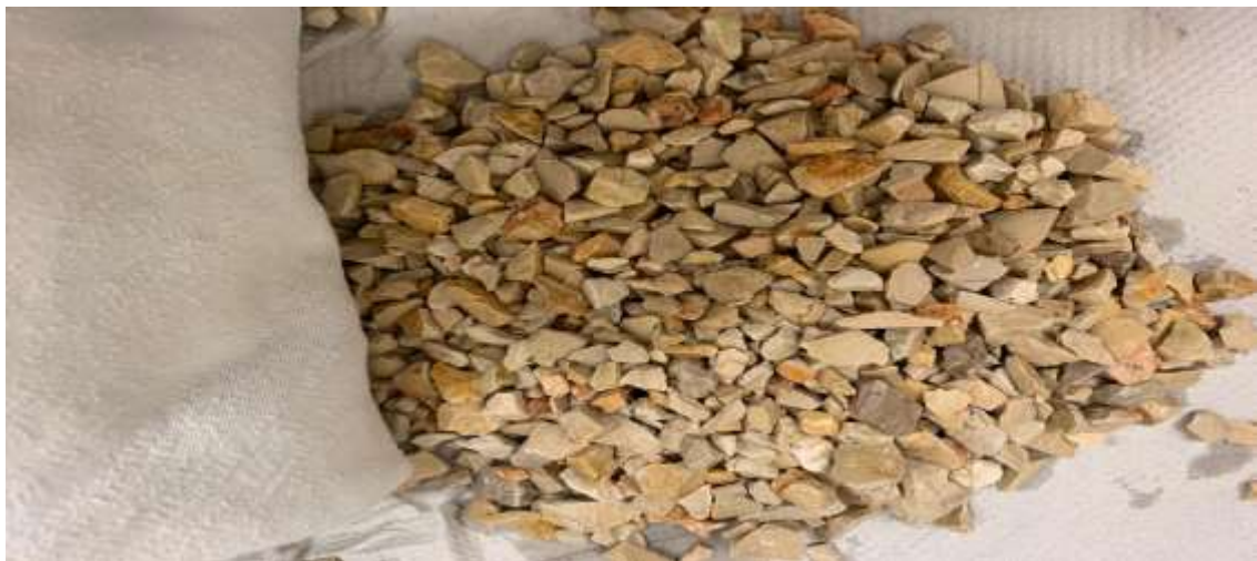
Figure 17. Removing surface water off aggregate using an absorbent clothing
