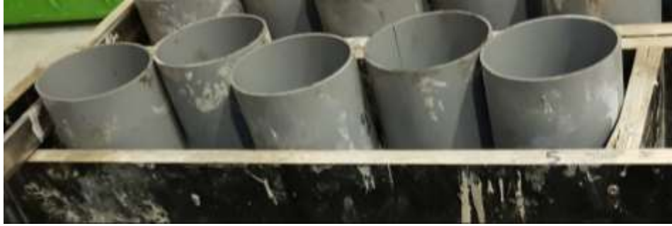
Figure 34. Compressive strength molds
