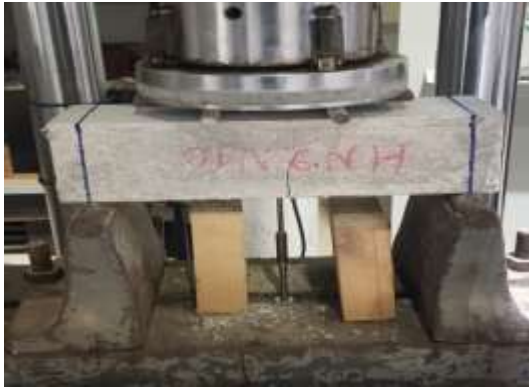
Figure 58. Flexural failure of mix with hemp
