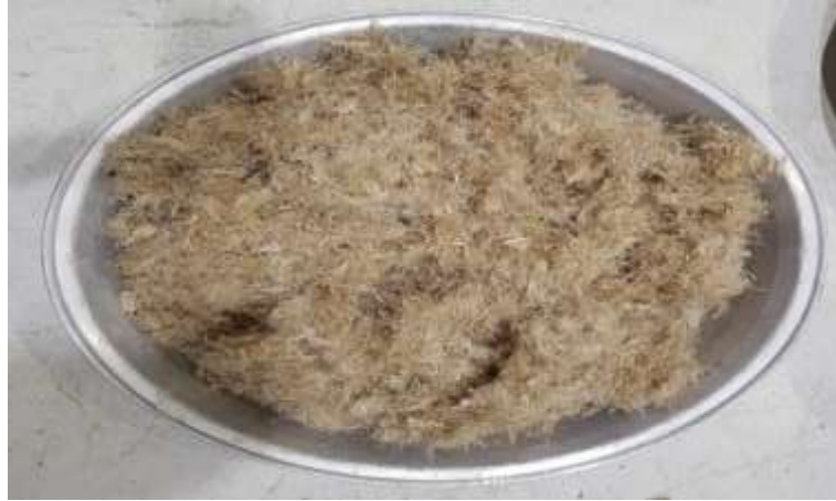
Figure 36. Dispersion of the hemp fibers.
