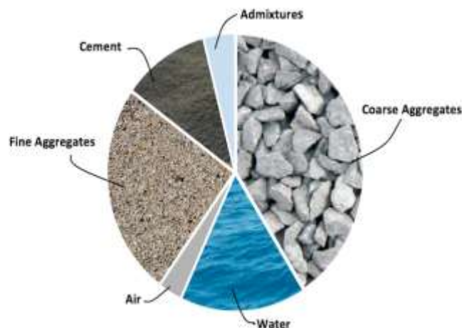
Figure 38. Constituents of the concrete mix
