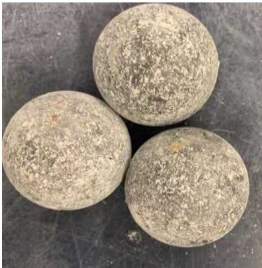
Figure 18. Steel balls of Los Angeles
