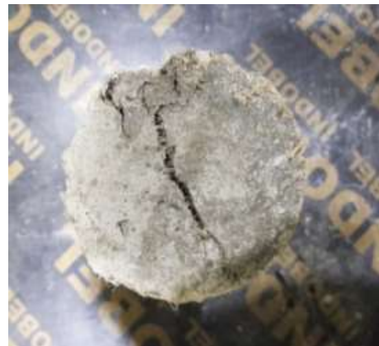
(c). Cracks bridging due to hemp
