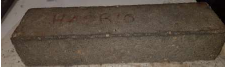
Figure 68. R20 and R10-H20-T1 specimens after 108 cycles
