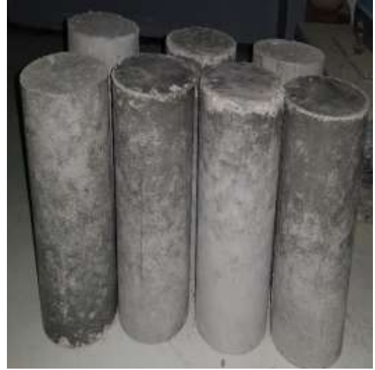
Figure 47. Compressive strength concrete specimen
