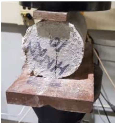
(b). Failure of hemp mix under tensile loads
