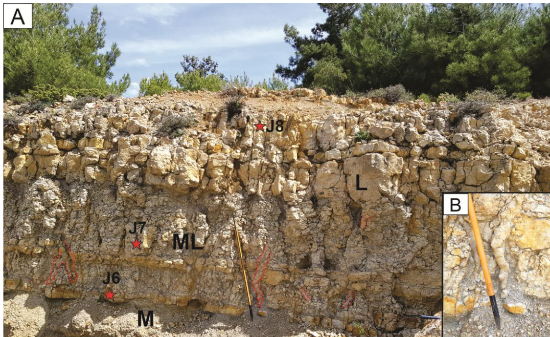
Figure 90: Field image of the burrowed marly limestone (ML) interval. Note the vertical change of facies from soft marls (M) at the base of the section to hard limestone (L) at its top. Note also the presence of vertical burrows cutting the horizontal strata (dotted red line). Samples J6, J7, and J8 were collected respectively from the base, middle, and upper part. B: Detailed photo of a vertical burrow cast.
