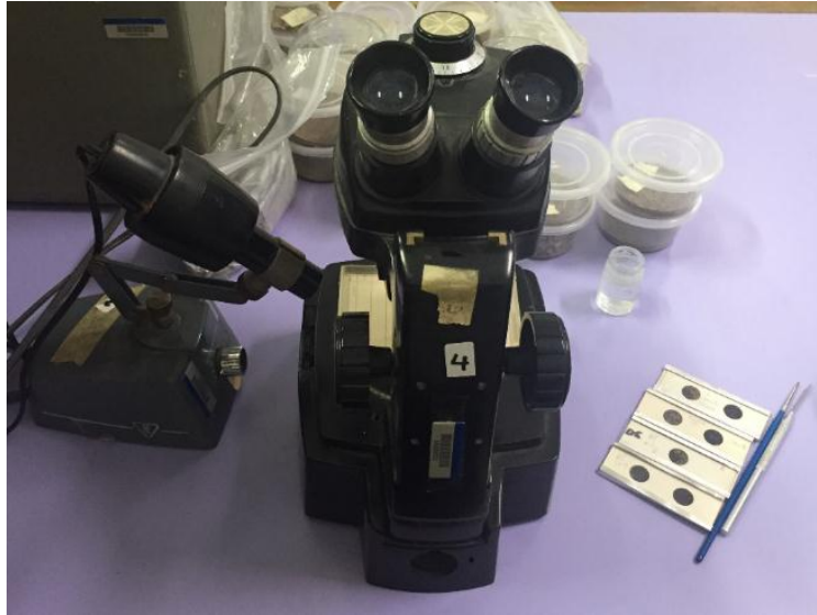
Figure 19: Binocular microscope, light, picking tray, brush, and microfossil cells used to store and study the microfossils.
