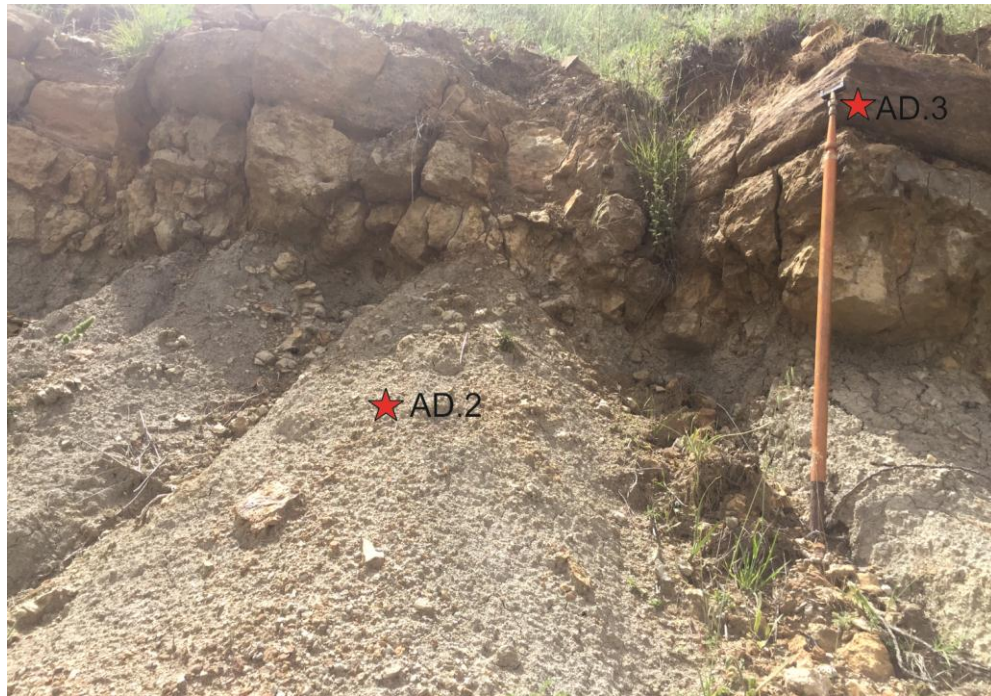
Figure 62: Field photo showing the location of samples AD.2 (dark grey marl) and AD.3 (grey limestone).
