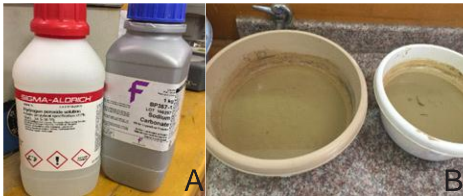
Figure 17: Sample preparation A: Chemicals used during the soft sample treatment (hydrogen peroxide and sodium carbonate), B: solution of the sample soaked with water and chemicals.
