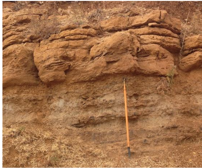
Figure 14: Jacob staff used to measure the thickness of beds (Barouk section).
