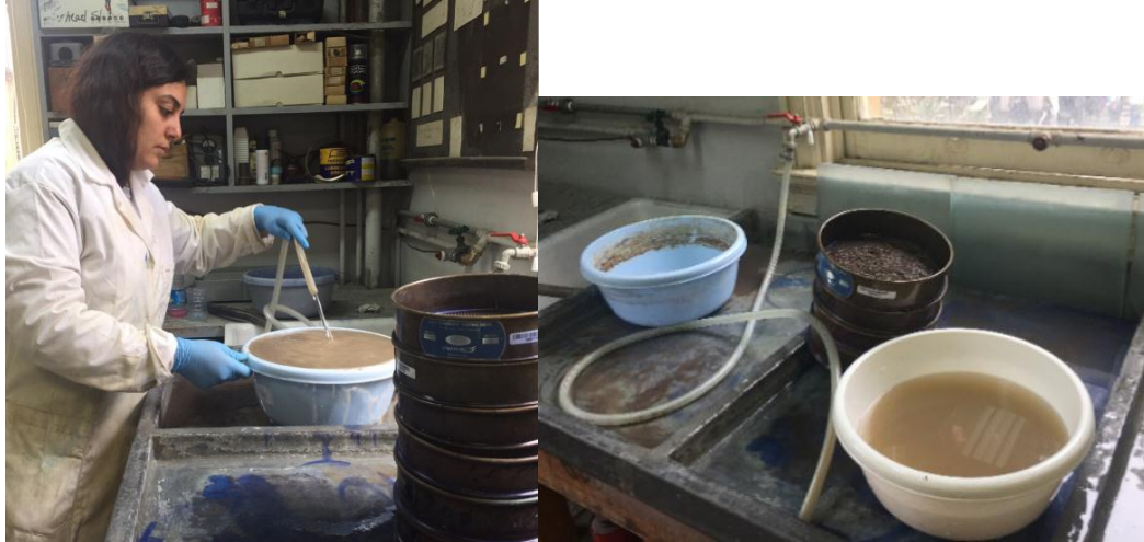
Figure 18: Sieving process of the soft rock samples for microfossil extraction. This process was performed in the thin section lab (Geology Department, AUB).
