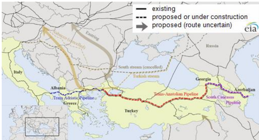
Figure 5 Major new transit pipelines from Russia and the Caspian Region to Europe.
