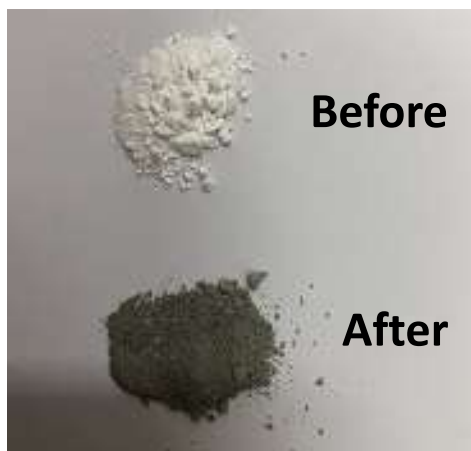
Figure 3.3. Photograph showing the color change of the UiO-66 before and after the loading of palladium.
