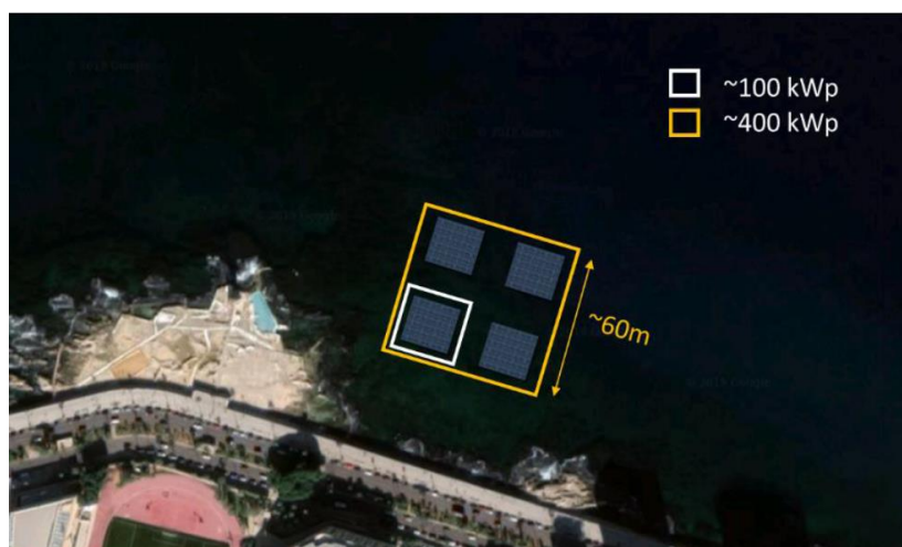
Figure 6-8: Potential layouts for SolarSea 4000 for the proposed two different system sizes (Swimsol, 2019).
