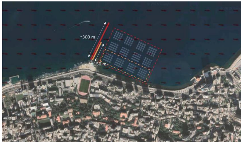
Figure 6-7: The layout of SolarSea 1500 with the proposed breakwater system on one side (Swimsol, 2019).
