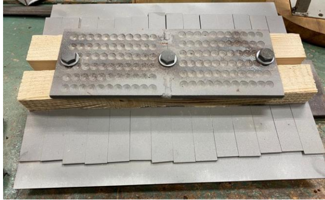
Figure 24. Sandblasted steel samples.
