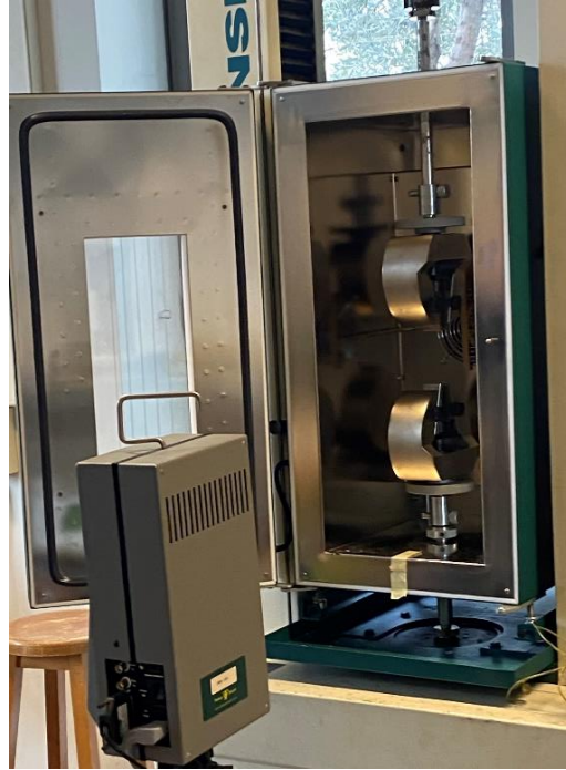
Figure 22. The Hounsfield H100KS universal tensile testing machine mounted with an environmental chamber and laser extensometer.
